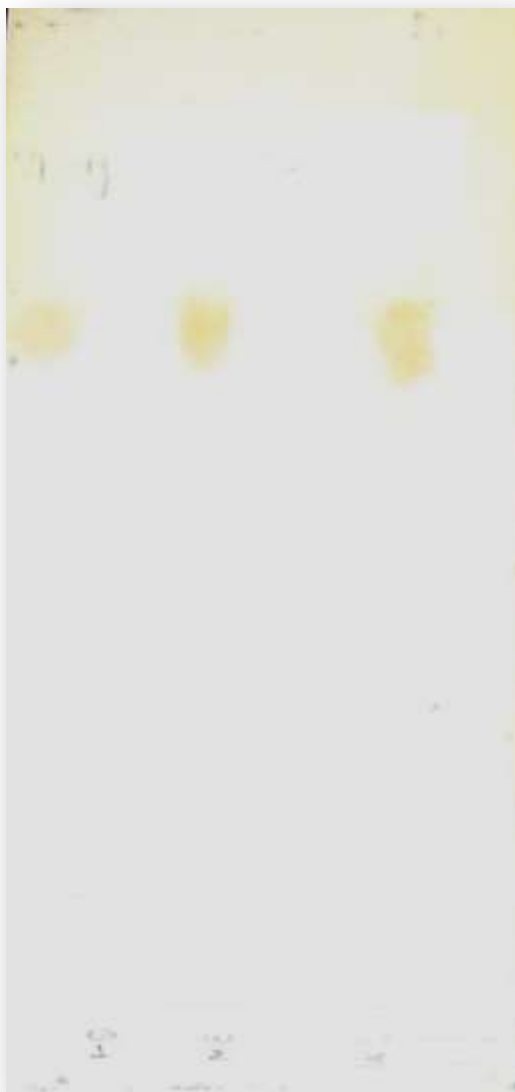
Figure -2: TLC analysis of flavonoids extracted by Harborne (1973). 1. Purified apigenin on Sephadex LH-20. 2. Crude apigenin .
