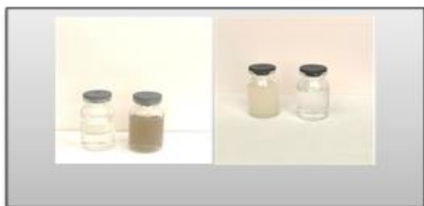
Figure 1. The color change during the synthesis of silver nanoparticles by the S. bouldardii . A- Silver nitrate solution + S. bouldardii solution after 1 hour. B- Silver nitrate solution only. C- Silver nitrate solution + S. bouldardii solution after 120 hours.
